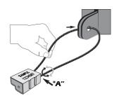
Pull the cable tight to the tightest aperture possible.
